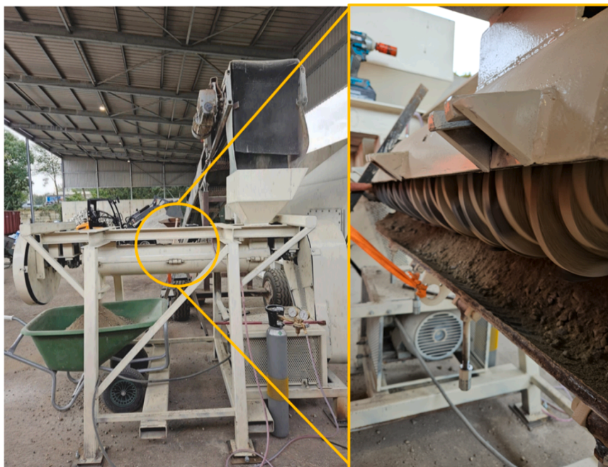
Fig. 4. Mangle, industrial-scale recycling technique for concrete.
