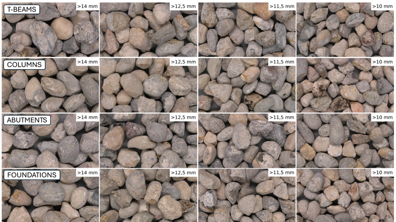
Fig. 7. Overview of the particle morphology of coarse RCA produced using the Smart Liberator.
