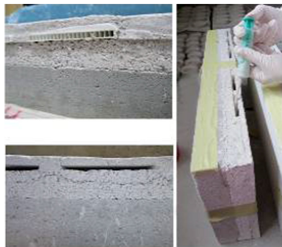
Fig. 10 Testing adhesion of grouts SIST EN 1015–12 (photo archive: A. Padovnik)
