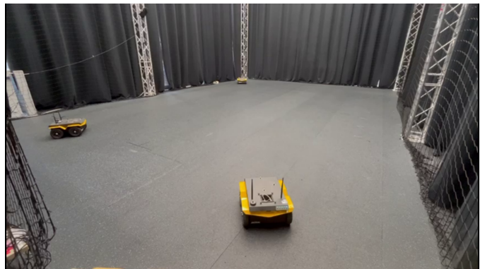
Fig. 13: Real-world R = 3 scenario, each robot performs an antipodal swap, moving across the arena to the opposite corner.
