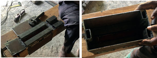
6. Weld the 3 rectangle tubes to the sides
