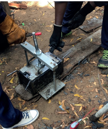
5. Pressing the mixture with a 14.7kN book press
