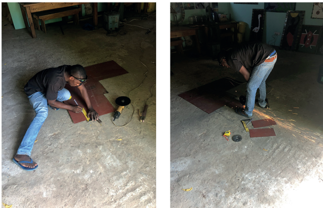
1. Cut the iron sheet in 6 pieces as shown above
