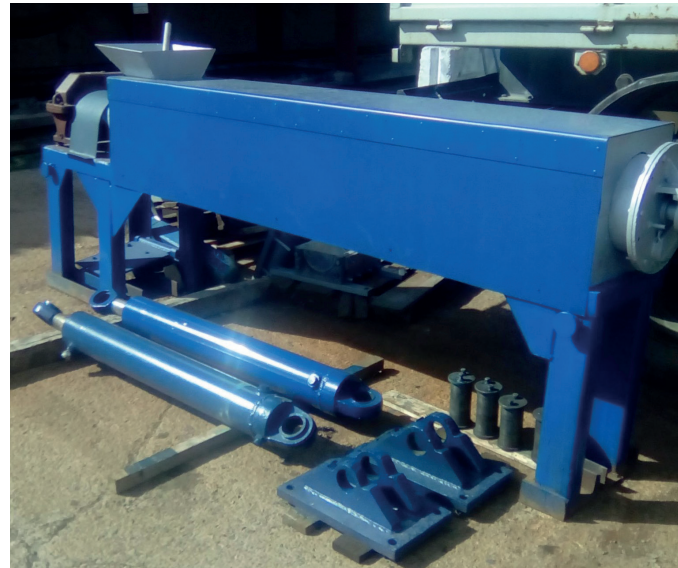
Figure 72. Exemplar plastic-sand extruder
