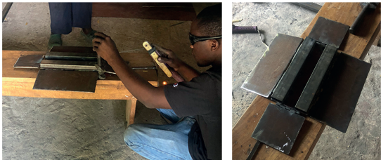
5. Weld the 2 rectangle tubes to the bottom
