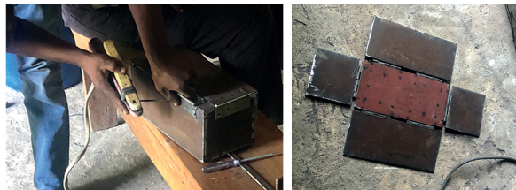
2. Weld the hinges to the sides and bottom to connect the parts
