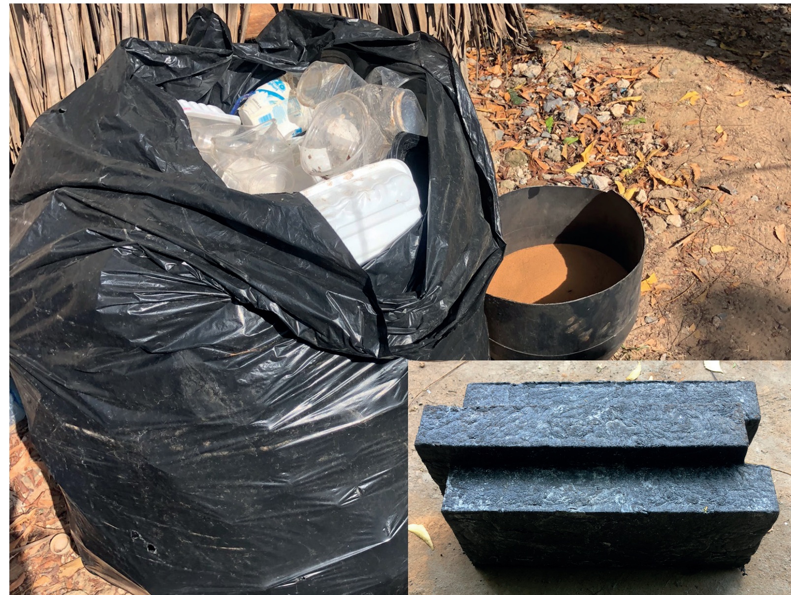
Figure 47. 3 kg of PP, 3 kg of sand and the final brick
