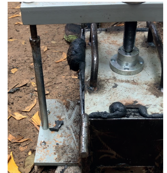
Figure 65. Plastic leakage in mould
