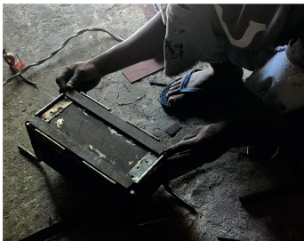
3. Weld pieces of metal to the bottom outside to make sure the hinges don't touch the ground
