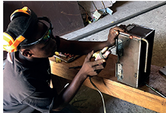
5. Weld the 8 small tubes to the 4 edges. 2 small tubes per edge
