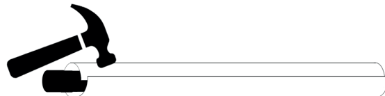
3. With a hammer hit the tube so it becomes the right size to fit around the rod
