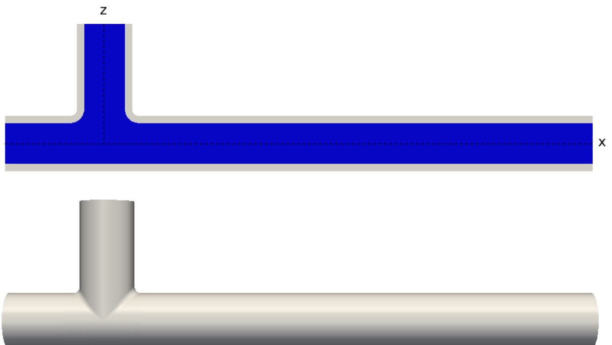
Figure 5.1.: The T-junction geometry. On top a section of the T-junction can be seen where the fluid has been coloured blue and the solid grey. On the bottom the outside of the T-junction can be seen.
