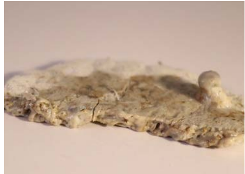
Figure 30: Heated by paint burner between plates
