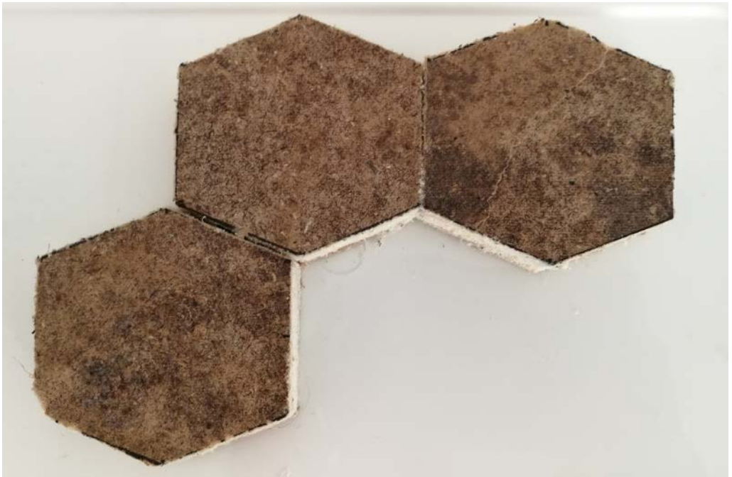
Ticking after pressing in a t-shirt press and cut into hexagons. Used during the interview with Merford.
