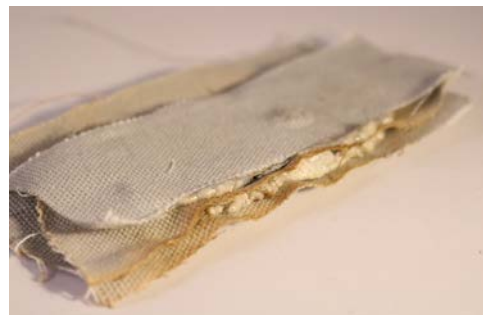
Figure 29: Molten inner layer, intact outer layer
