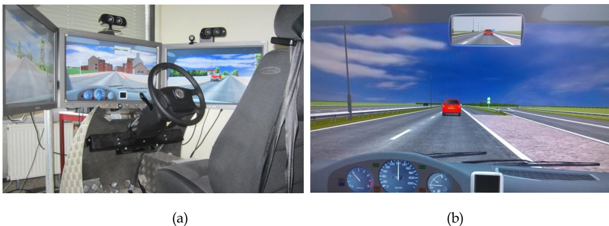
Figure 2.1: (a) The medium-fidelity fixed-based driving simulator and (b) the driving simulation environment in the two-lane freeway.
