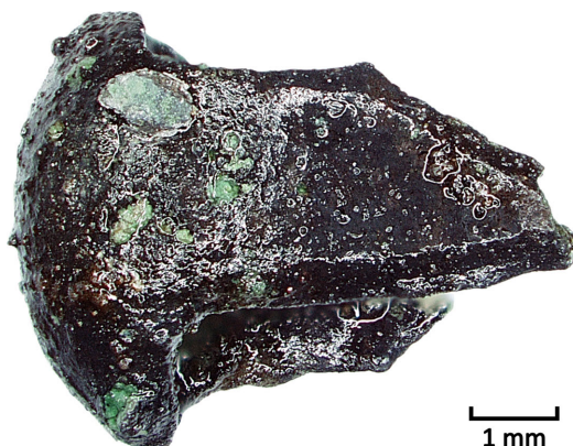
Fig. 5.4: Black regions on the studs are characterized by tenorite. Green malachite grains are also observed on this particular stud. Optical micrograph.
