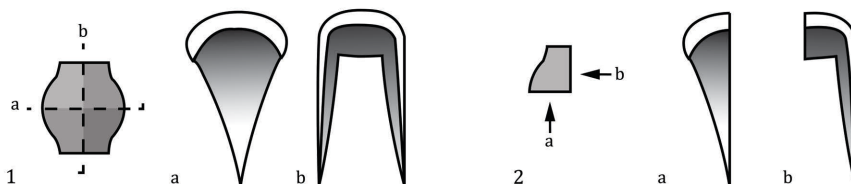
Fig. 2.2: Indication of the sectioning process, creating cross-sections of the leg and the intact stud (Table 2.1). (1) Top view of sectioning of (embedded) specimen along line a and b (side views of subsequent cross-section); (2) resulting quarter of a stud with respective side views. Reproduced from Nienhuis et al. 2013, Fig. 9.13.
