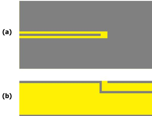
**Figure 3.7:** (a) Top and (b) side view of the stripline-to-CPW transition. On the left side, the CPW is in metal layer M6, with the ground plane being metal layer M1, on the right side, the stripline is inside the silicon oxide on metal layer M5.
