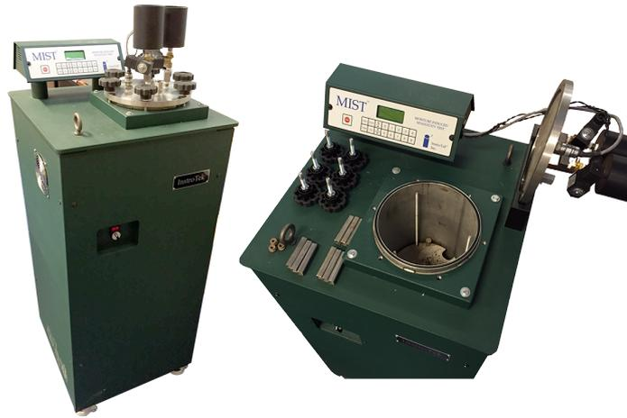
Figure 3.1: Moisture induced Sensitivity Tester
