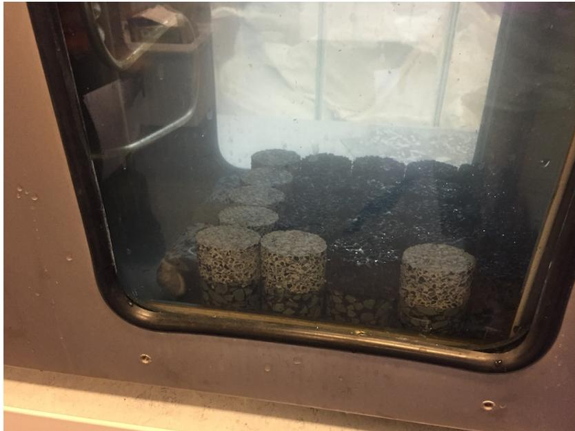
Figure 5.2: Cores in the conditioning bath. Note that two cores of Mixture B are orientated in a different direction. This is because the raster of cores was what kept the cores upright. Since those 2 were not in the raster, they were placed flat so that they would not wobble around by the currents in the bath.
