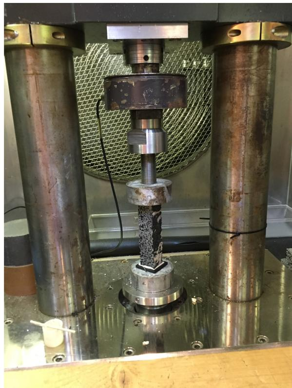
Figure 6.1: Test setup for determination of cohesive strength
