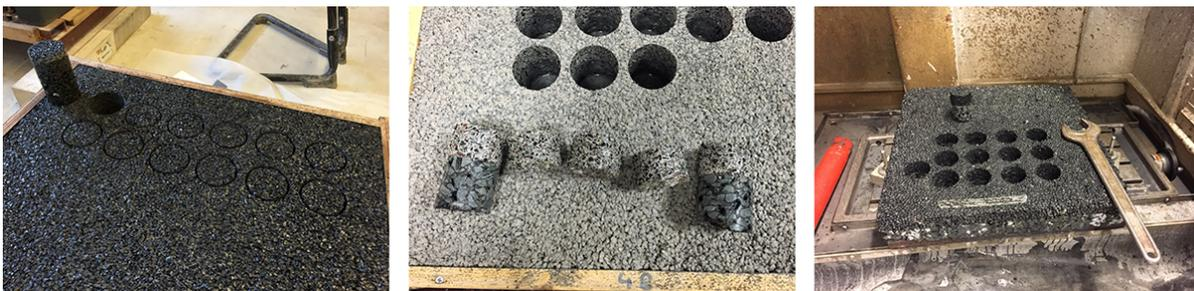
Figure 5.1: The 3 mixtures after coring the 50mm cores.
