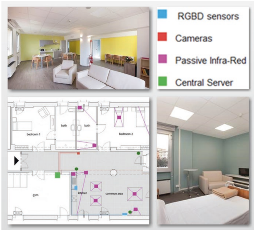
Fig. 5.1 Architectural and sensor design in the ‘smart home’ of the MODIPRO project [24]
