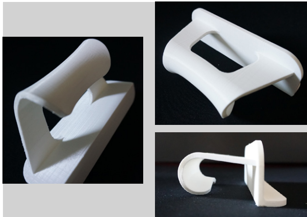
Modeled and 3D printed hook
