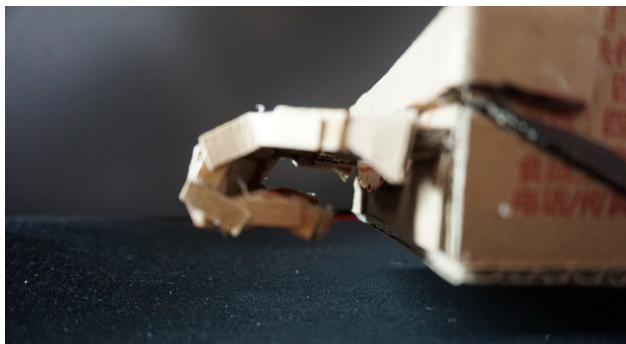
Cardboard prototype of hook and kit body
