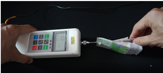
Force test using force gauge
