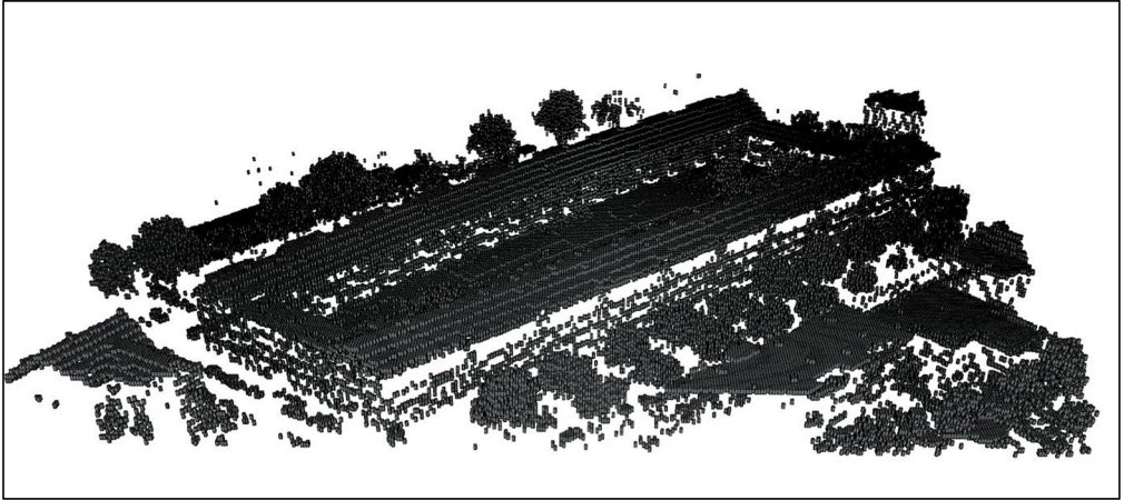
Fig. 5. Rotterdam AHN-2 dataset, Noordereiland, voxel count 81,588, 0.4\text{m} \times 0.4\text{m} \times 1\text{m} .
