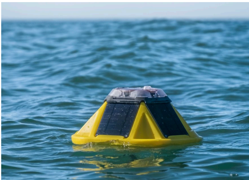
Figure 4.5: The Sofar Ocean Spotter buoy used for marine environmental monitoring. The buoy is solar-powered, transmits data via satellite or cellular networks, and supports additional Smart Mooring sensors for current and water-quality measurement (Source: Sofar Ocean, 2025).
