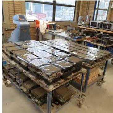
(b) Plastic sheet cover on concrete cubes for 24 h immediately after casting
