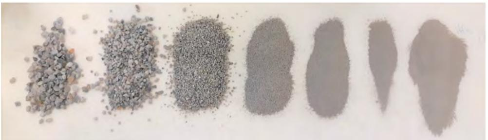
Figure 3.8: Various fractions of fRCA NC - From left to right :  $>4$  mm, 1-4 mm, 0.5-1 mm, 0.25-0.5 mm, 0.125-0.25 mm,  $<0.125$  mm.
