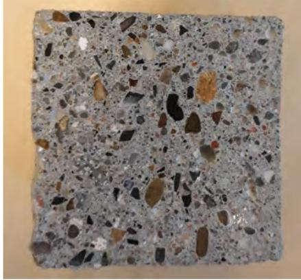
Figure 3.13: Polished section of a mortar mixture of Series 1
