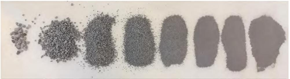
Figure 3.7: Various fractions of fRCA NB - From left to right :  $>4$  mm, 2-4 mm, 1-2 mm, 0.5-1 mm, 0.25-0.5 mm, 0.125-0.25 mm,  $<0.125$  mm.
