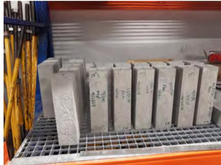
(b) Curing and storage of concrete specimens for shrinkage at  $20^\circ\text{C}$  and 55 % RH
