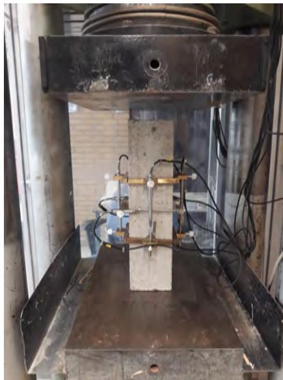
Figure 3.18: Experimental setup for elastic modulus tests of concrete
