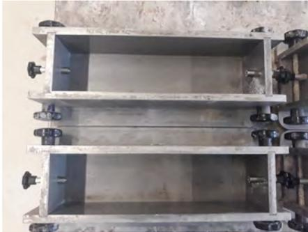
(a) Shrinkage molds of  $75 \times 75 \times 280 \text{ mm}^3$
