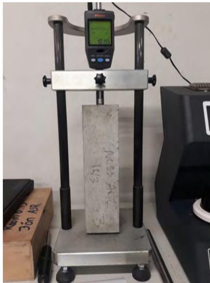
Figure 3.20: Measuring gauge device for shrinkage of concrete
