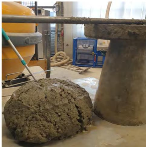
Figure 3.15: Slump test set up for fresh concrete mixtures
