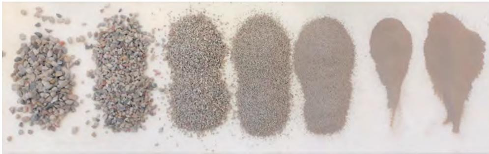
Figure 3.9: Various fractions of fRCA ND - From left to right :  $>4$  mm, 1-4 mm, 0.5-1 mm, 0.25-0.5 mm, 0.125-0.25 mm,  $<0.125$  mm.
