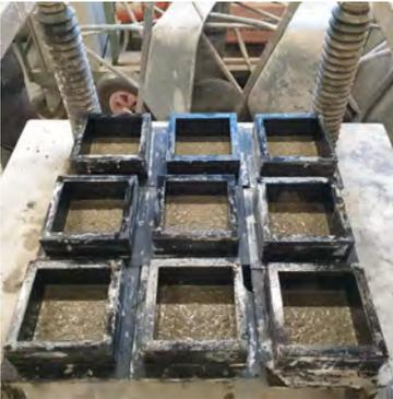
(a) Introduction of freshly mixed concrete in two layers
