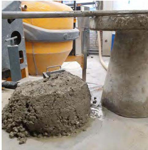
Figure 4.19: Stable concrete mixture after slump testing
