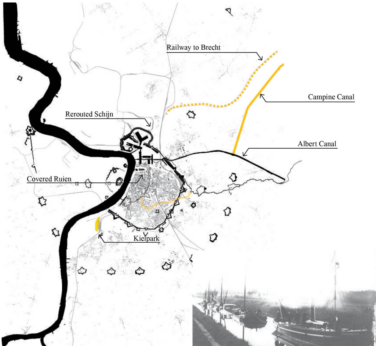
FIGURE 3 Situation between 1850 and 1950 (map). The Ruien were entirely covered and integrated into the municipal sewage system, evacuating waste water in the Scheldt River. Waste was transported to the countryside via the Campine Canal (1885-1916) (picture) and railway network.
