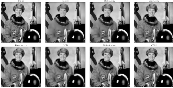
Fig. 2. A ResNet with varying convolutions is overfitted to a target image created with twenty anisotropic diffusion steps. DeltaConv can reproduce the filter well, where other convolutions struggle. (Courtesy NASA)
