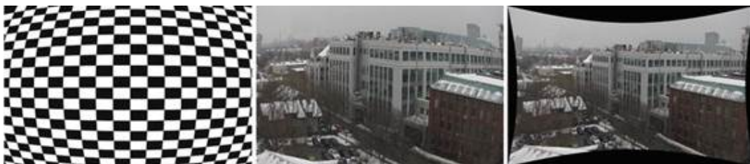
Figure 2.15: Radial distortion (Image taken from [11])
