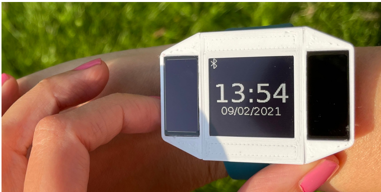
Figure 5.1: First battery-free open-source [73] smartwatch with FreeBie: intermittently-powered bi-directional BLE link.
