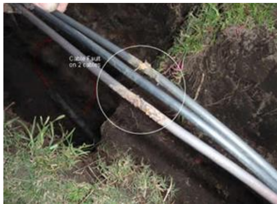
Figure 4.7: Cable damage- short circuit condition
