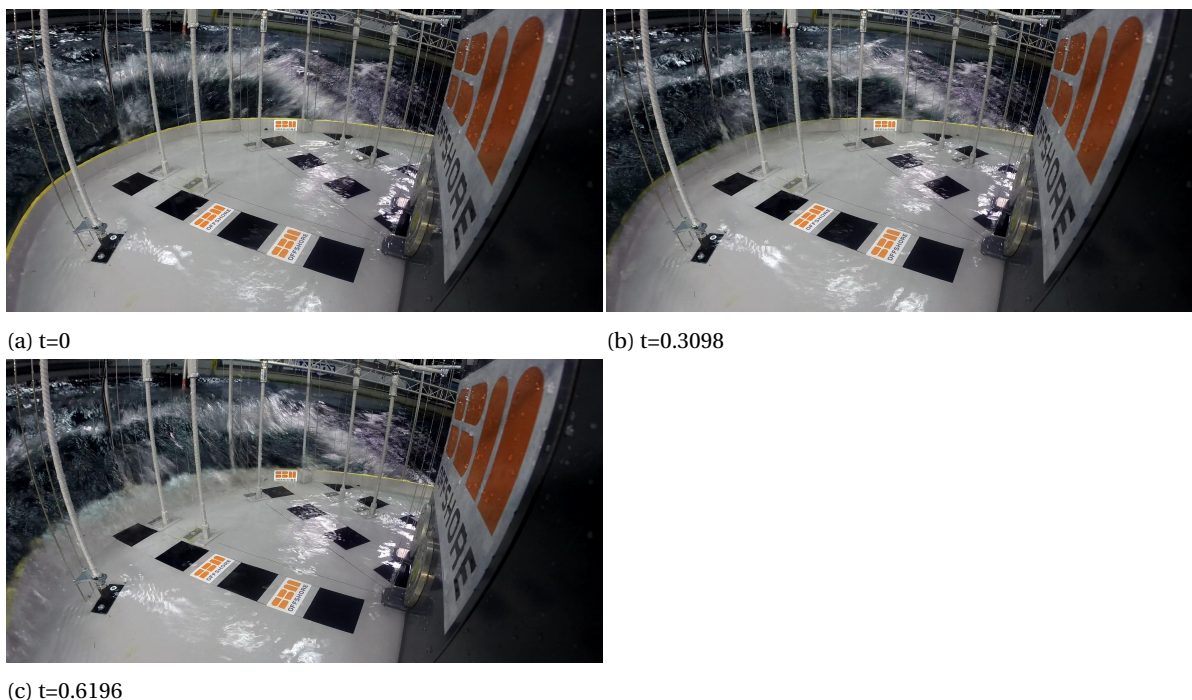
Figure 4.9: Frame by frame footage of a green water wave flowing on deck, with a frame-rate of 25 frames per second
