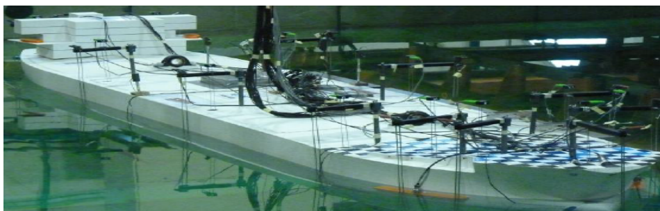
Figure C.2: Spread moored model test with water on deck sensors ( Veer and Zuidscherwoude [2012] )
