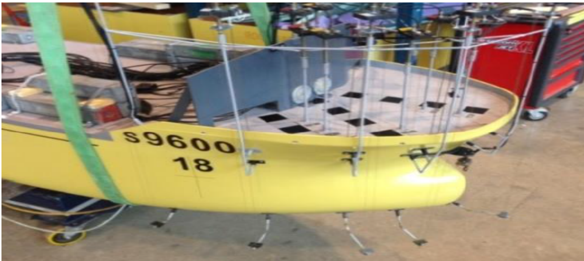
Figure 3.3: Location of the sensors on the bow, photo of actual model
