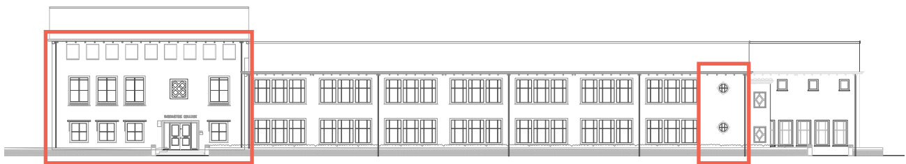
Figure 46 Load-bearing walls south facade
