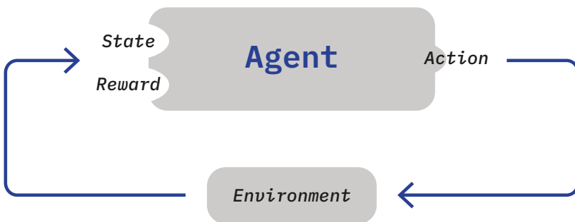
Figure 4.3: A schematic of a typical reinforcement learning algorithm from adapted Sutton and Barto (2018).
