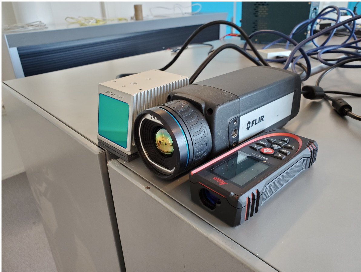
Figure 2.21: Sensor setup showing from left to right the Livox LiDAR, FLIR IR camera and a laser range-finder for the ground-truth distance
