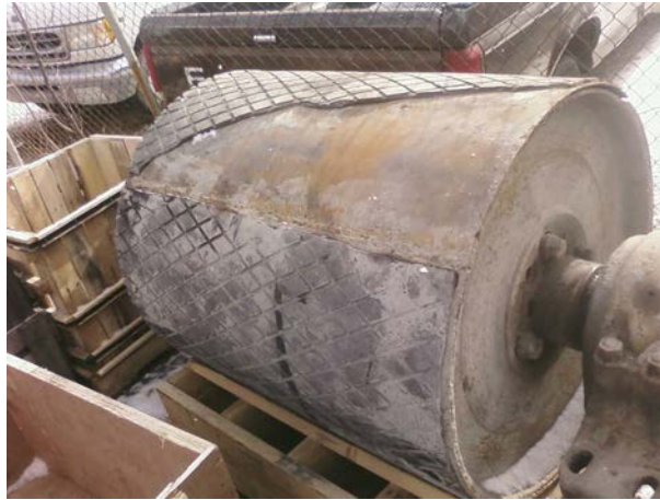
Figure 3.6: Pieces of a head pulley's rubber lagging were frequently torn loose due to the belt slippage around the drive pulley. Courtesy of Belzona (2016).
