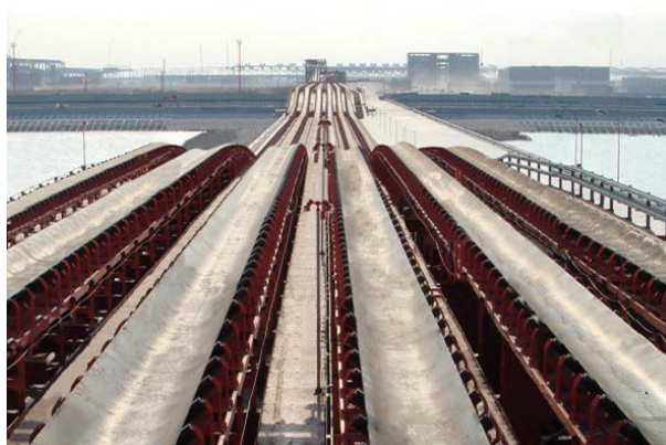
Figure 1.1: Belt conveyors in Shanghai Port, Luojing Phase II ore terminal. (Courtesy of Shanghai Keda Heavy Industry Group Co., Ltd. (KDHI, 2016))
