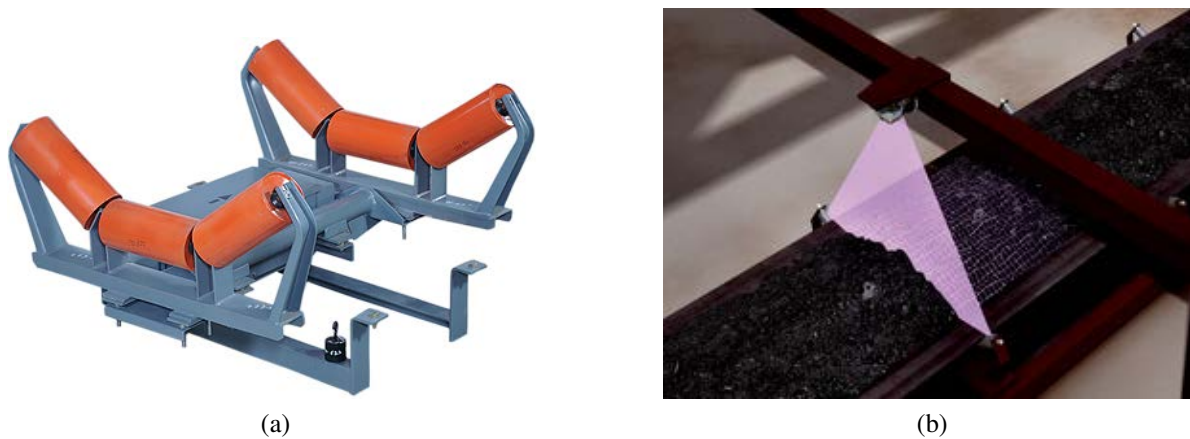
Figure 2.5: Material flow sensors. (a) Belt scale, courtesy of FLSmidth Pfister Limited (2017). (b) Laser profilometer, courtesy of SICK B.V. (2017).
