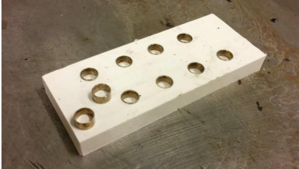
Figure 4. Silicon mold, with stainless steel rings in place during preparation of bitumen specimens.
