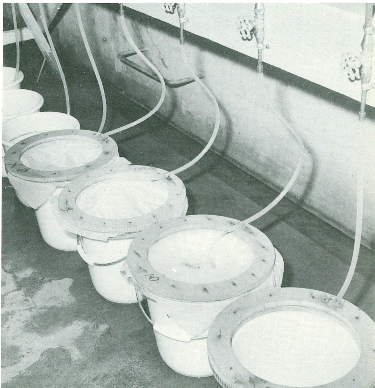
2. Separation of water and sediment by means of filter material ( mesh size = 50 \mu\text{m} )
