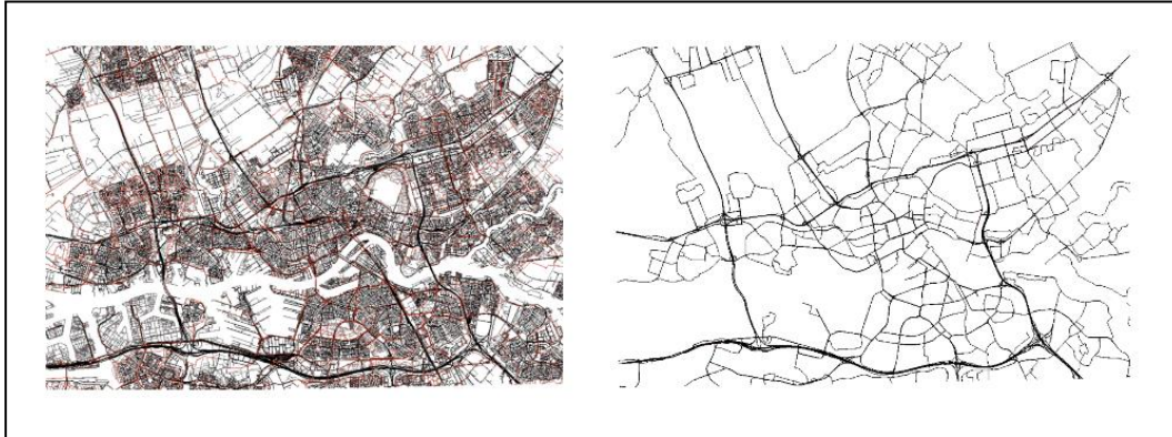
Figure 4. 5. Side by side comparison of the OSM network before and after the filtering
