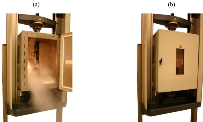
Figure 5.6: Pull-out test setup for the -20 , +60 and +80^{\circ}\text{C} test series; photographs of the test setup; (a) The climate box was cooled to -20^{\circ}\text{C} with vaporized liquid nitrogen (the door was closed during the test); (b) The climate box was heated to +60 and +80^{\circ}\text{C} with an electric heating element (not visible on the photograph).
