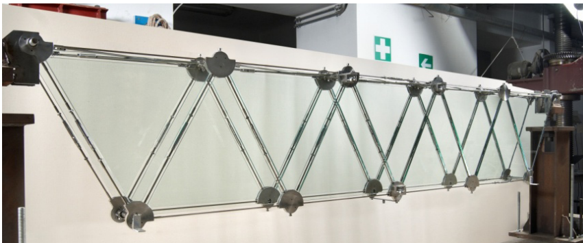
Figure 3.19: Steel-glass hybrid beam Froli & Lani [Froli & Lani, 2010a, b].
