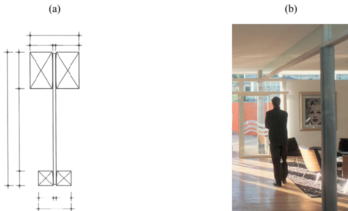
Figure 3.24: Timber-glass beams investigated by Hamm & Kreher
