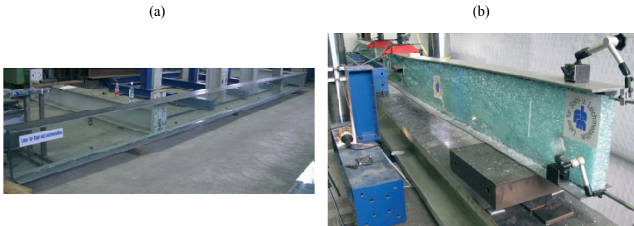
Figure 3.13: Steel-glass hybrid beam investigated by Bucak & Bues [Bucak et al., 2009 a, b].
