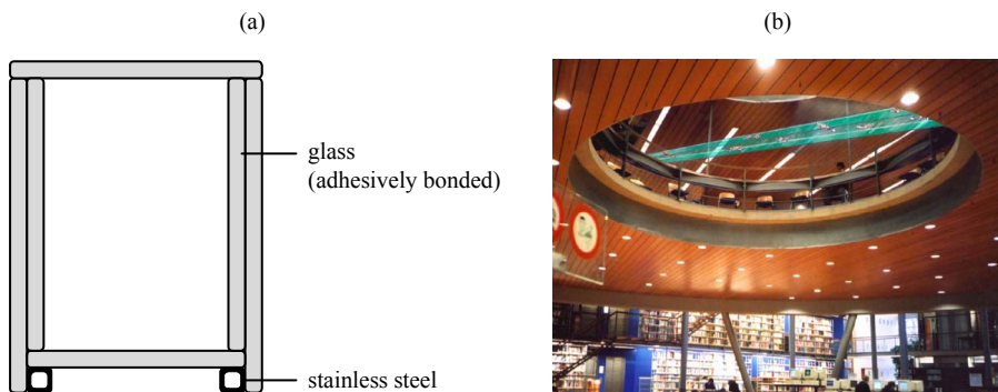
Figure 3.3: Reinforced glass box-section aquarium [Veer et al., 2003b]; (a) schematic representation of the cross-section of the aquarium; (b) artist impression of the 8 m aquarium suspended in the air.
