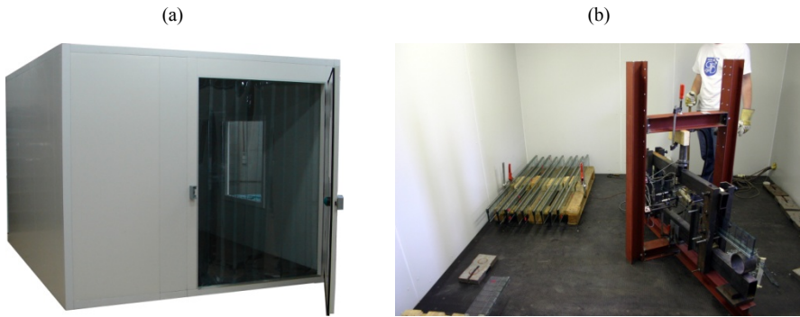
Figure 5.10: Bending test setup at +60°C, within a climate chamber.
