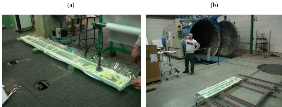
Figure 10.3: (a) The assembled reinforced glass beam in a vacuum bag, prior to lamination; (b) two 1.5 m beam specimens in vacuum bags ready to enter the autoclave (in the back).
