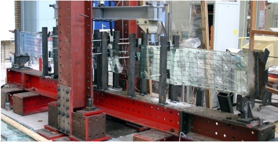
Figure IV.6: Post-tensioned glass beam buckled at right beam end.
