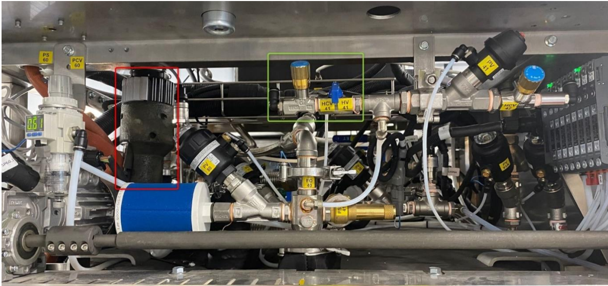
Figure 6. The NCG (red square) and needle valve (green square) installed on the sterilizer.
