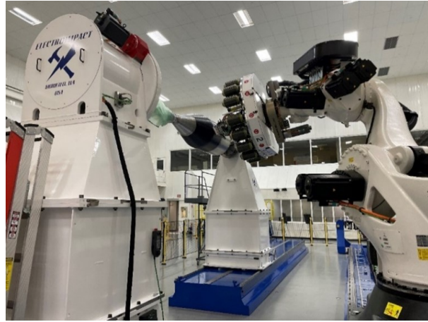
Figure 3.11: Test article being manufactured with the MSFC AFP robot.
