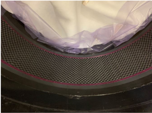
Figure 4.5: Close up image of the reinforcement after cure.
