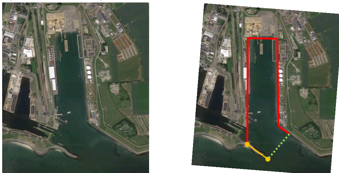
Figure 4.13: Left: aerial picture of the 'Vlissingen Buitenhaven'; right: schematization of the geometry in the empirical model (red = quay walls, orange = closure dam, green dotted = harbour entrance, rotation of the geometry of 5 degrees for practicality reasons)
