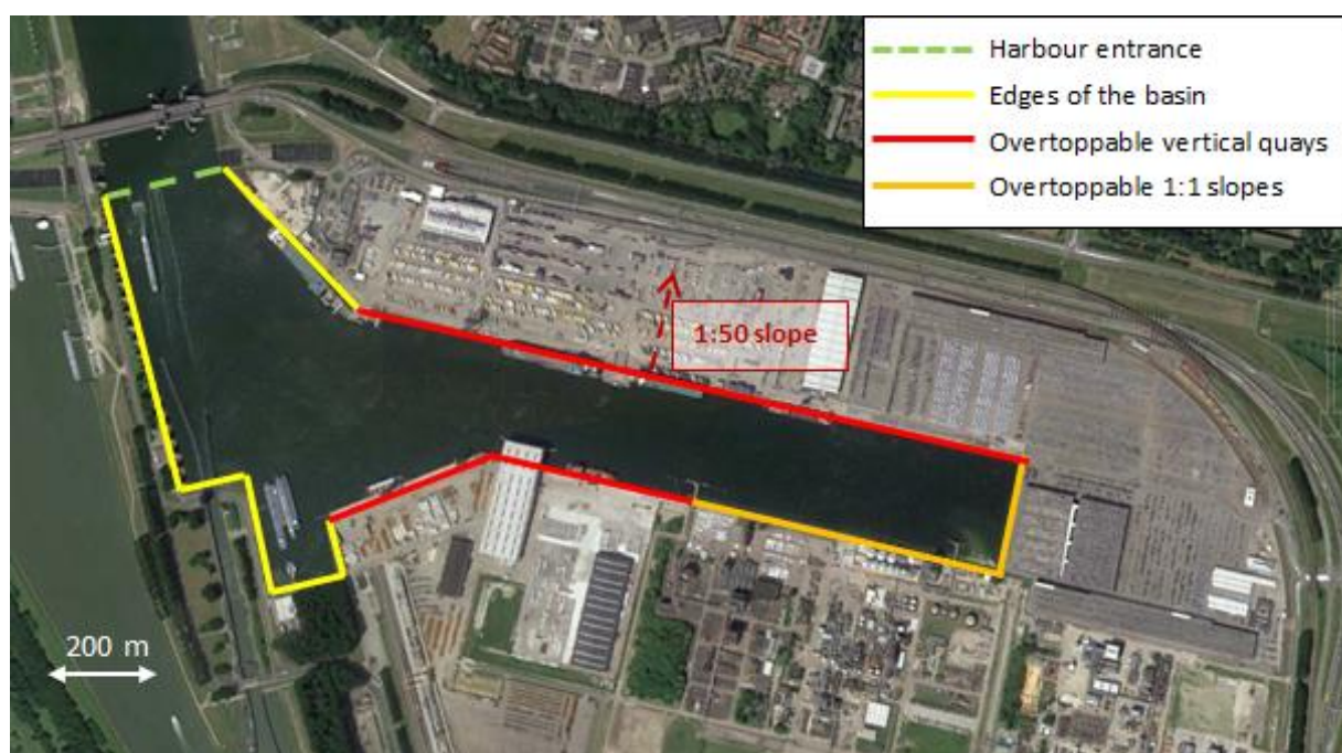
Figure 5.4: Schematization of the Brittaniëhaven with a background of an aerial picture of the area.
