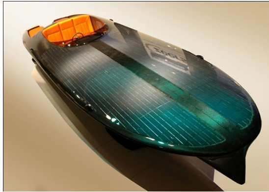
Figure 14: PV powered boat 'Czeers MK1' with horizontal PV placement in the hull (2007).
