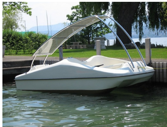
Figure 11: SOL10; typical PV powered recreation boat build by KOPF AG, Germany.
