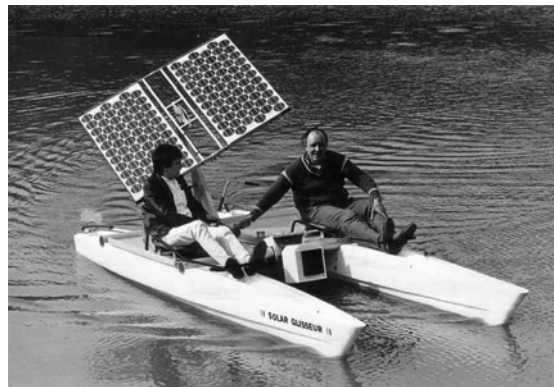
Figure 15: PV powered boat 'Solar Glisseur' with adjustable PV; One of the first solar powered boats (1984).
