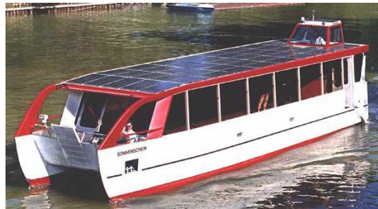
Figure 10: Sonnenschein; typical PV powered people's transportation boat build by SUEK GmbH, Austria.
