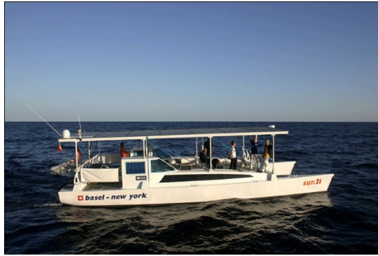
Figure 12: Sun21; Typical PV powered boat for private/research purposes. Used to cross the Atlantic Ocean, build by Swiss transatlantic21 Association (2007).
