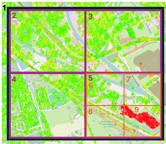
Figure 8.2.: Example of quadrant classification, starting with the large black quadrant (1). Due to the additional subsidence signal in the bottom right (a newly installed solar farm), this quadrant is further subdivided into four new (purple) quadrants. Quadrants 2, 3, and 4 contain only one deformation phenomenon and will not be further subdivided, whereas quadrant 5 will be split into four new sub-quadrants. This way, areas exhibiting local shallow and autonomous signals are isolated from areas only representing the deep deformation signal.
