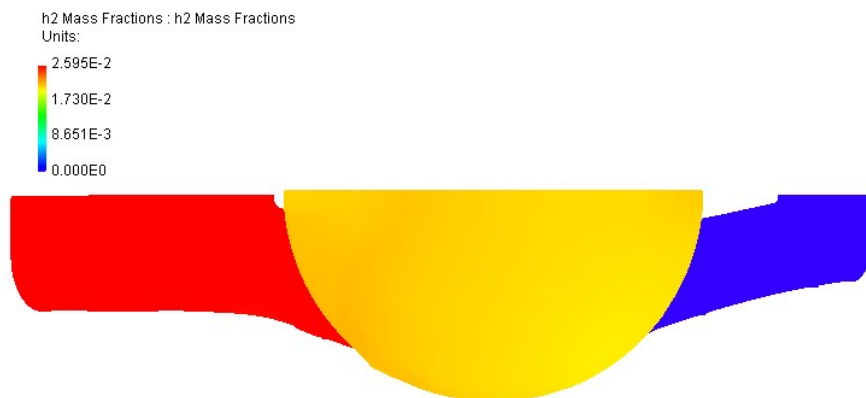
Figure 6.42: Bottom view of the hydrogen distribution at 5 degrees BTDC, using indirect hydrogen injection
