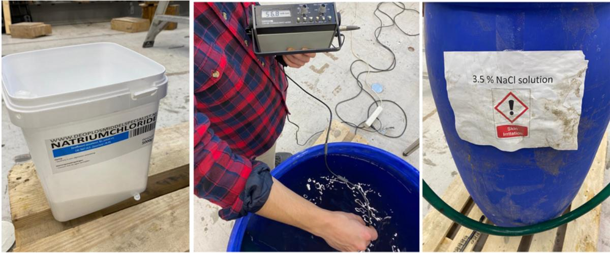
Figure 3.6: Production of artificial seawater and salinity test (middle)
