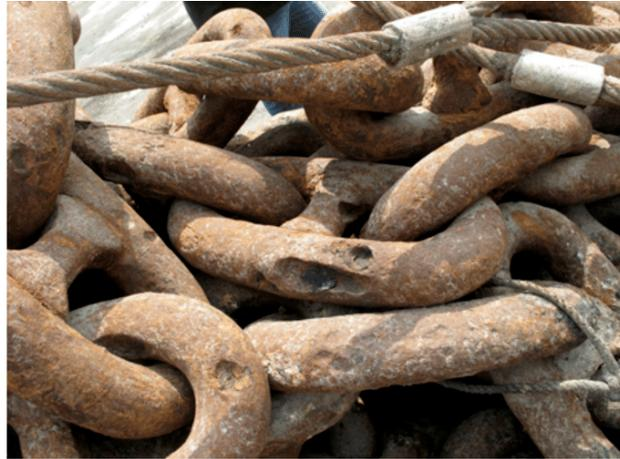
**Figure 1.3:** Local attack of corrosion [12]
