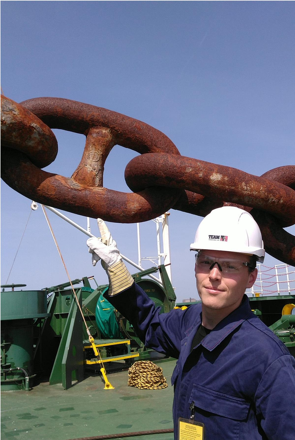
Figure 5.1: Visual inspection of full-scale mooring chain of the MARAN ARES.
