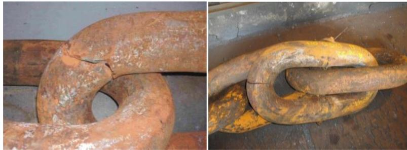
Figure 1.5: Fatigue in mooring chain [18]
