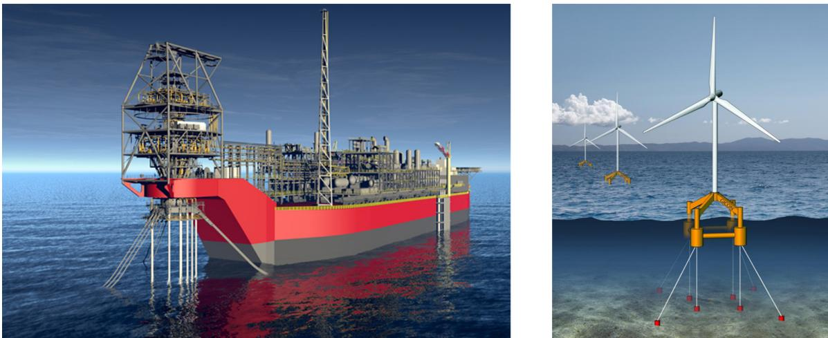
Figure 1.1: Floating structures with mooring chains, [1],[2]
