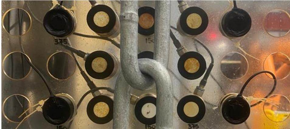
Figure 3.11: 9 Vallen AE sensors and 4 hydrophones.
