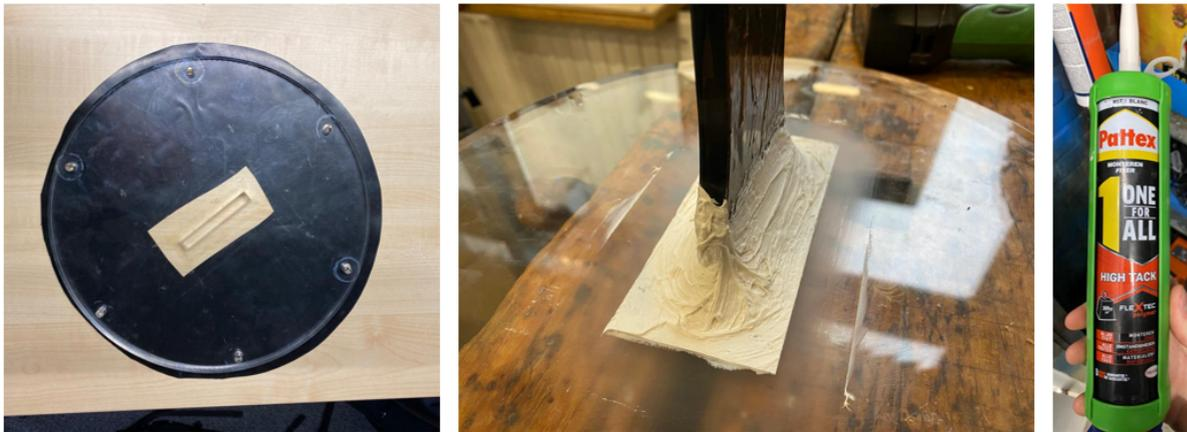
**Figure 3.3:** Connecting the specimen to the connector disc.
