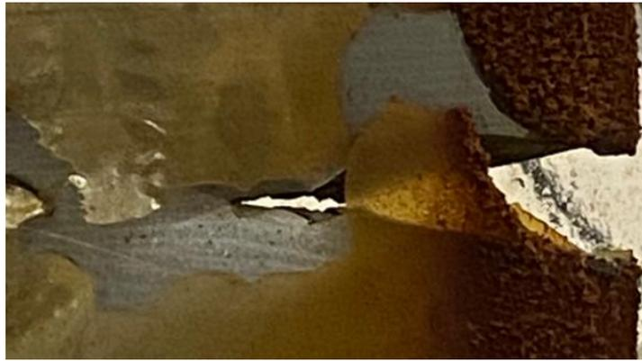
**Figure 4.12:** Final crack of failed sample 3.
