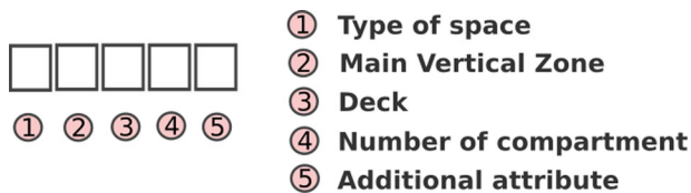
Figure 2. Structure of the input for spaces.
