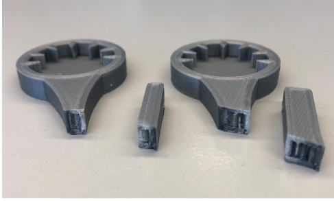
Figure 5.4: Break point in concept 1 (left) and concept 2 (right). Figure 5.5: Deformation of the pin and broken lever teeth.
