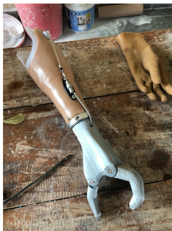
Figure 2.9: 100 Dollar hand, a 3D printed mechanical prosthesis with metal linkage mechanism, attached to locally produced socket in India.
