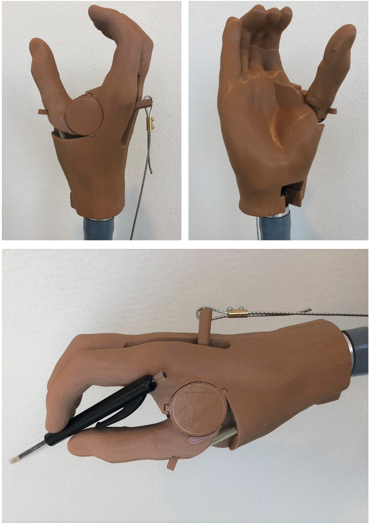
Figure 4.9: The final design of the 3D-Sanhand: the 3D printed Simple to Assemble Natural-looking hand prosthesis.
