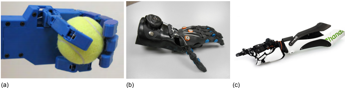
Figure 1.2: Different examples of hand prostheses created with AM technology: a) Gosselin's hand; a body powered under-actuated prosthetic hand [25], b) Cyborg Beast; a body powered prosthetic hand prosthesis for children [26], c) Handiii CYOTE; an externally (myoelectric) powered forearm prosthesis [27]
