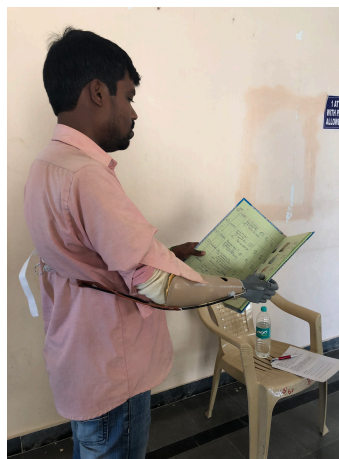
Figure 2.9: 100 Dollar hand, a 3D printed mechanical prosthesis with metal linkage mechanism, attached to locally produced socket in India.
