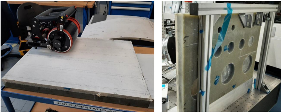
Figure 6.13 The flat glass fiber-reinforced polymer plate with 50 mm thickness.
