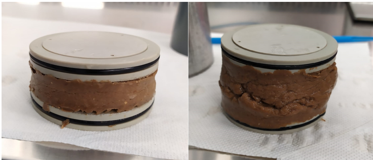
Figure 4.6: This is a picture taken of a successful dewaterability experiment with a well-formed sludge cake (left) and of a poorly formed sludge cake (right)
