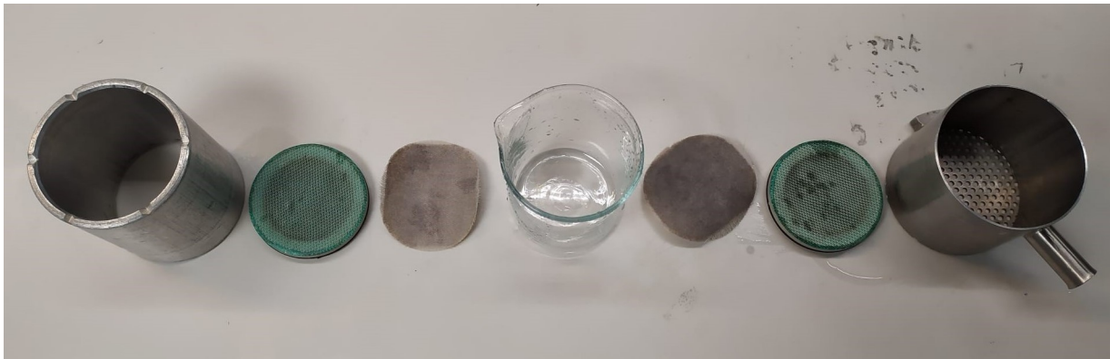
Figure 3.3: Overview of the Mareco chamber filter press and its components. From left to right: beaker (with grooves upward to prevent spillage), filter disc, support filter, sample, support filter, filter disc, beaker holder
