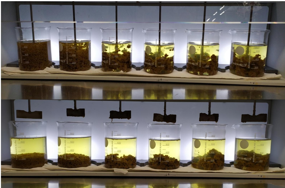
Figure 4.3: First jar test to determine the ideal C-2230 dose when the samples are pre-treated with an ideal PAX-18 dose of 2.0 ml/l with samples from the vacuum toilet. The uppermost picture was during the mixing phase and the bottom picture was after two minutes of settling. The respective dosages of C-2230 from left to right were: 10, 15, 20, 25, 30, and 35 ml/l
