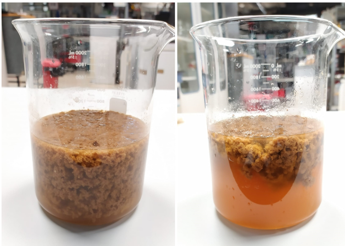
Figure 4.7: Flocculation with a low amount (70 ml/l) of C-2230 (left) and with a high amount (150 ml/l) of C-2230 (right). Photo was taken of both sludges from the experiment in Table 4.8
