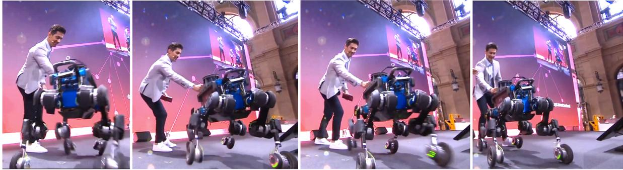
Fig. 6. ANYmal on wheels reacting to external force disturbances from a human. The inverted pendulum term in foothold predictions helps to guide the placement of the feet to recover balance.
