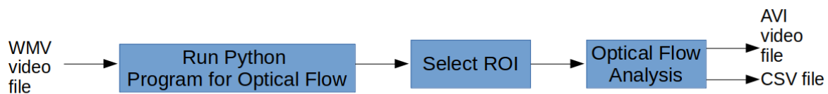
Figure 3.8: Optical Flow analysis of IR camera recordings
