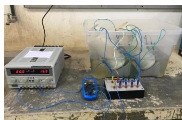
Figure 2: Chloride chloride migration test in progress
