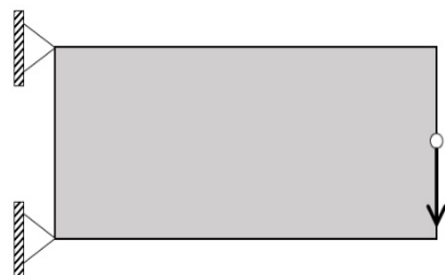
Figure 9. Cantilever beam boundary conditions.
