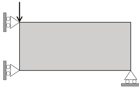
Figure 5. MBB symmetric beam and boundary conditions.
