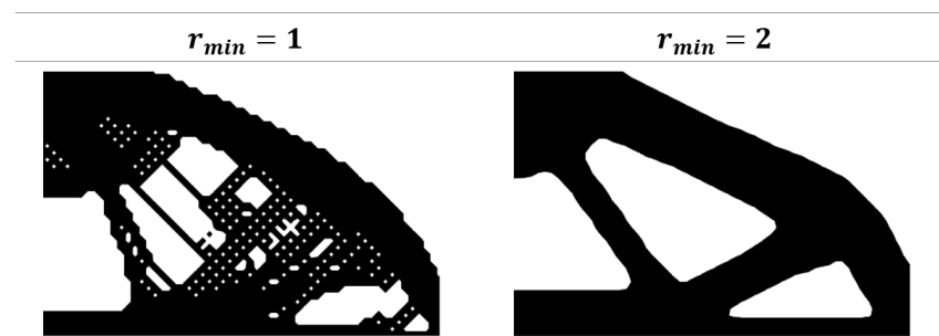
Figure 1. Effect of using filter radius ( r_{min} ) on optimum topology.
