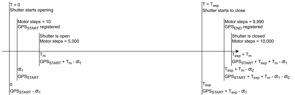
Figure 3.5: Time sequence of the shutter. The steps between events are not to scale.
