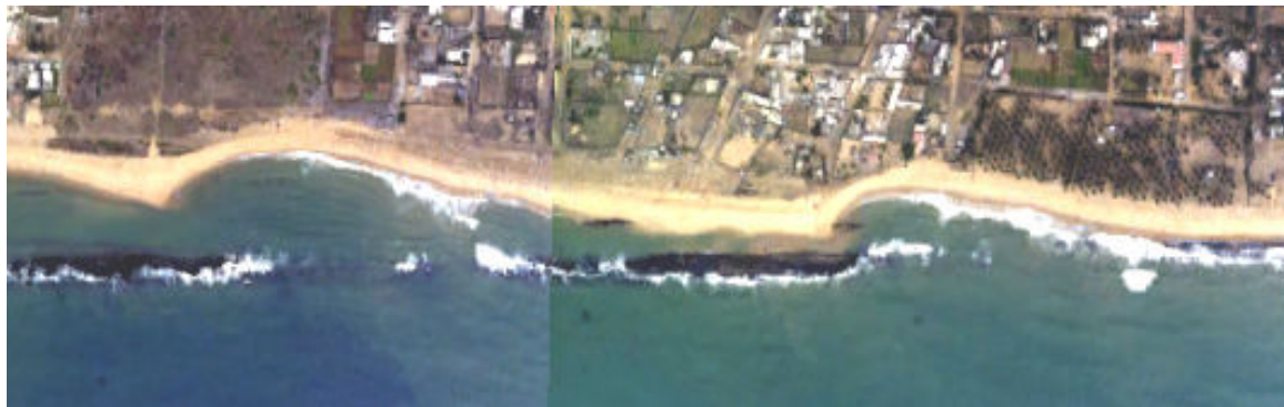
Figure 37 Asymmetrical erosion profiles. Further erosion progression from right gap is blocked by the presence of beachrock behind the main formation.
