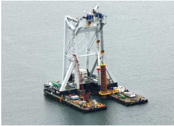
Figure 2: Svanen 10,000mt lifting capacity (LondonArray)
