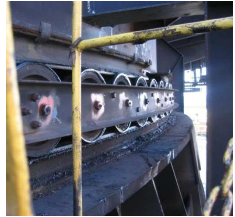
Figure 30: Outer slew bearing rollers Thialf
