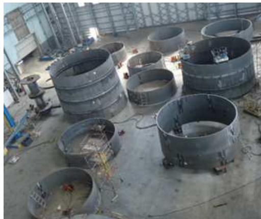
Figure 35: Ring sections of mast Aegir (HMC)
