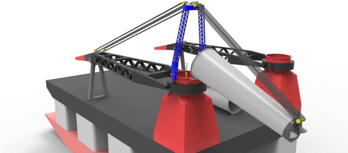
Figure 85: Back-mast concept with two tackles
