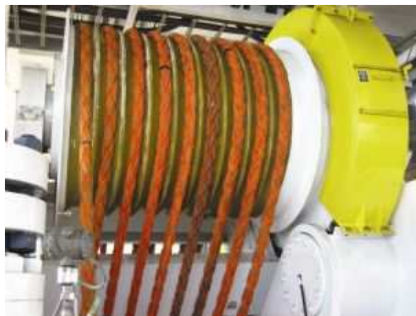
Figure 10: Synthetic rope on traction winch
