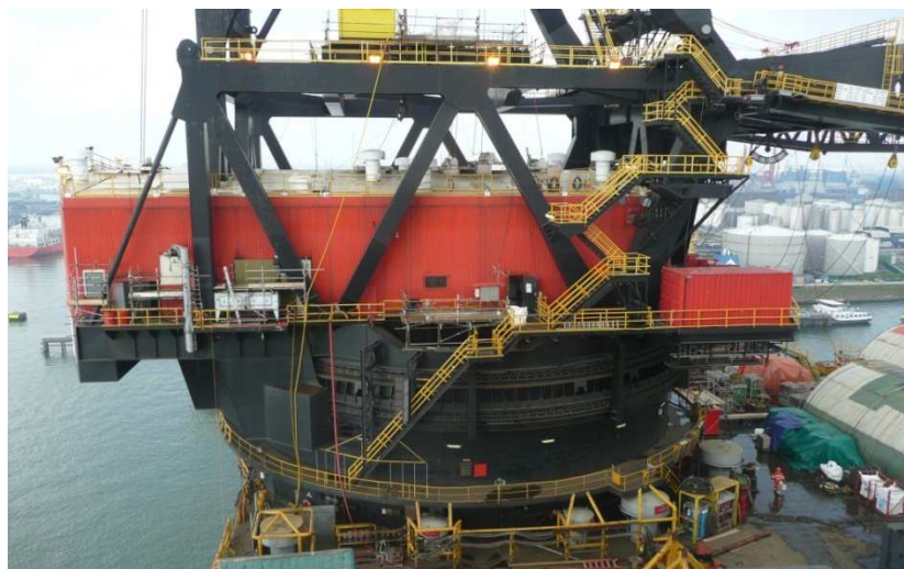
Figure 39: Circular footprint of an A-frame crane with roller slew bearing (HMC)
