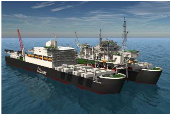
Figure 4: Pieter Schelte, topside lifting system (Setcorp)
