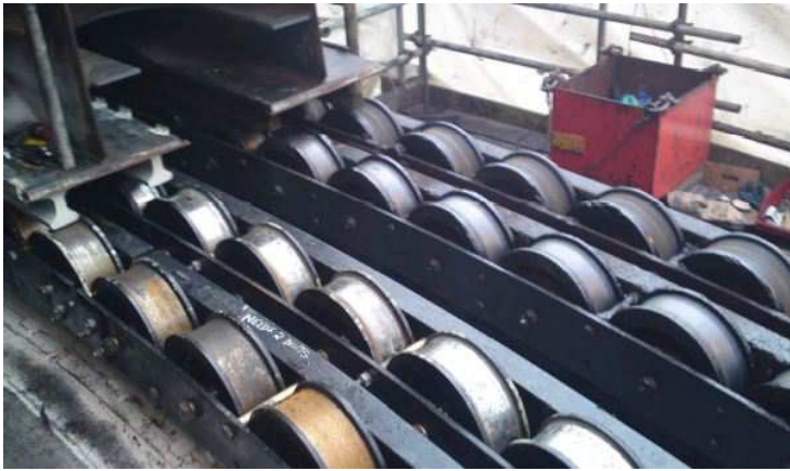
Figure 29: Top view slew bearing rollers Thialf
