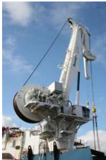
Figure 122: Knuckle boom crane with drum at the tail (Huisman)
