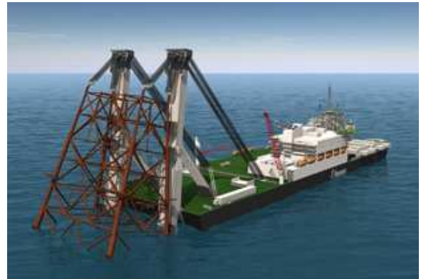
Figure 5: Pieter Schelte, jacket lifting system (Deltamarin)
