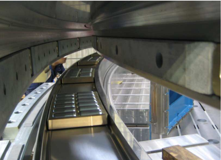
Figure 32: Slew bearing jacked up, showing the Orkot pads, race plates and cage sections (HMC)
