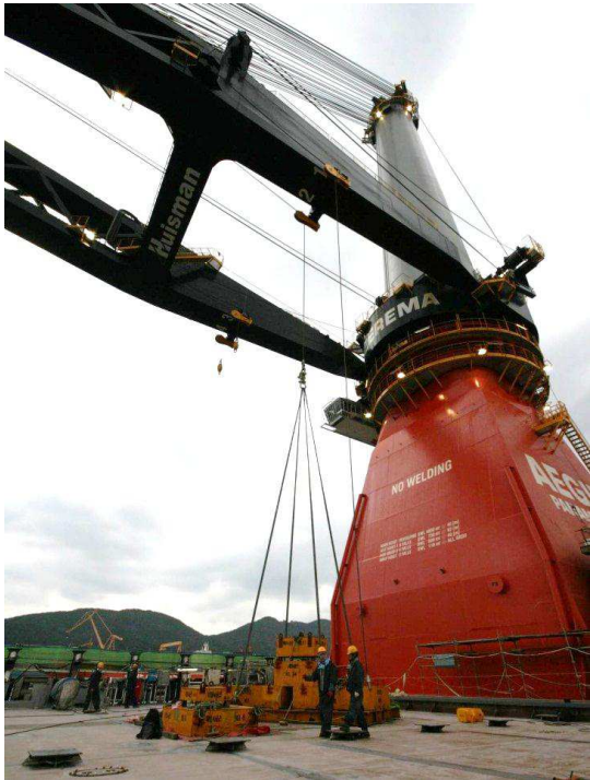
Figure 40: Square footprint of a mast crane (HMC)
