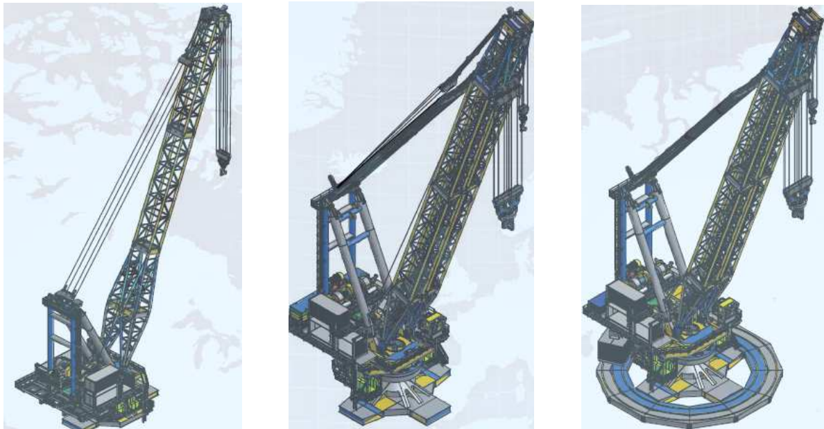
Figure 117: Ringer multi-crane with a long single boom (left), a heavy duty boom (center) and a ringer attachment (right) (Zwagerman)
