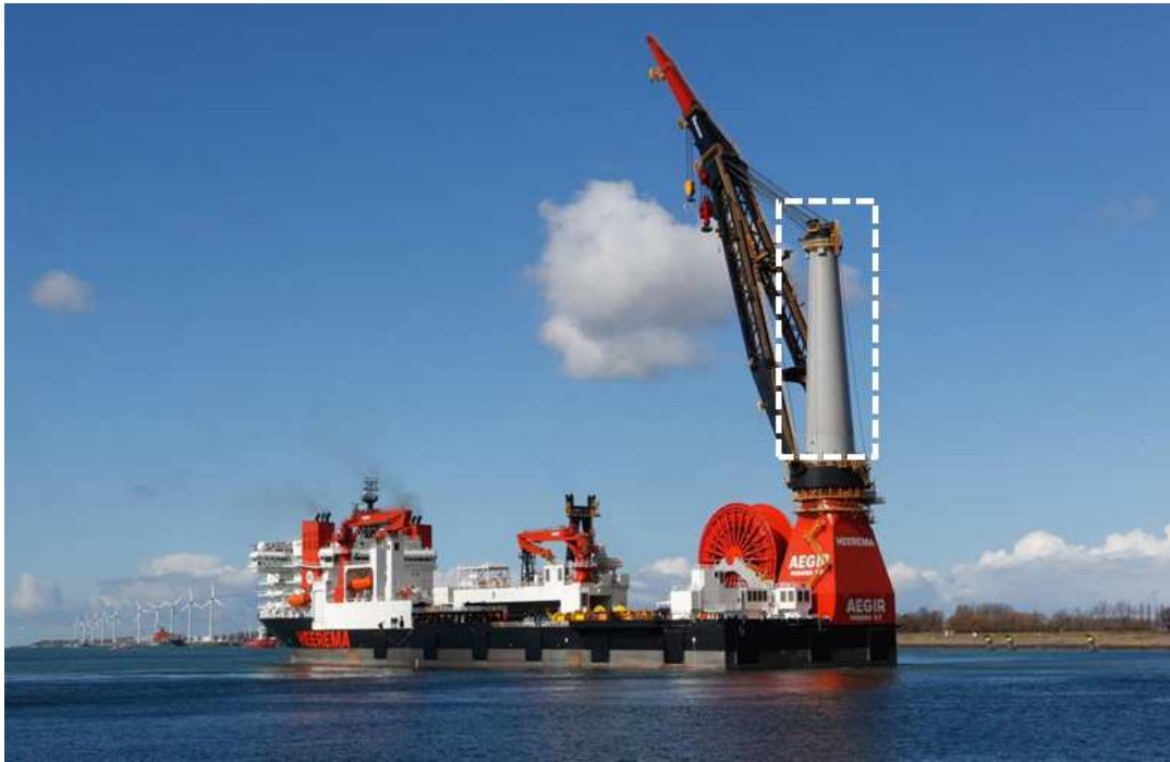
Figure 55: Mast section to be removed (HMC)
