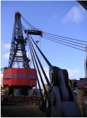
Figure 36: Boom tie-back mode
