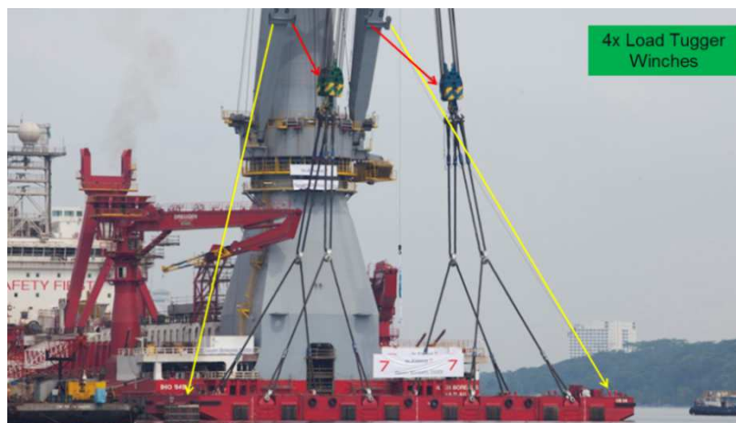
Figure 51: Load tuggers on Seven Borealis (HMC)
