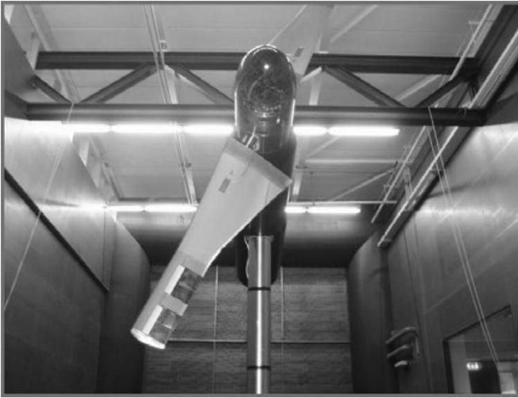
**Figure 3.2** – “Smart” rotor scale model in the Open Jet facility (van Wingerden, Hulskamp, Barlas, Houtzager et al., 2011).
