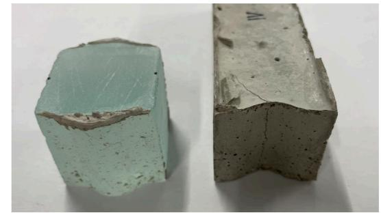
Interfacial failure + Concrete failure
