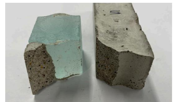
Serrated interfacial failure
