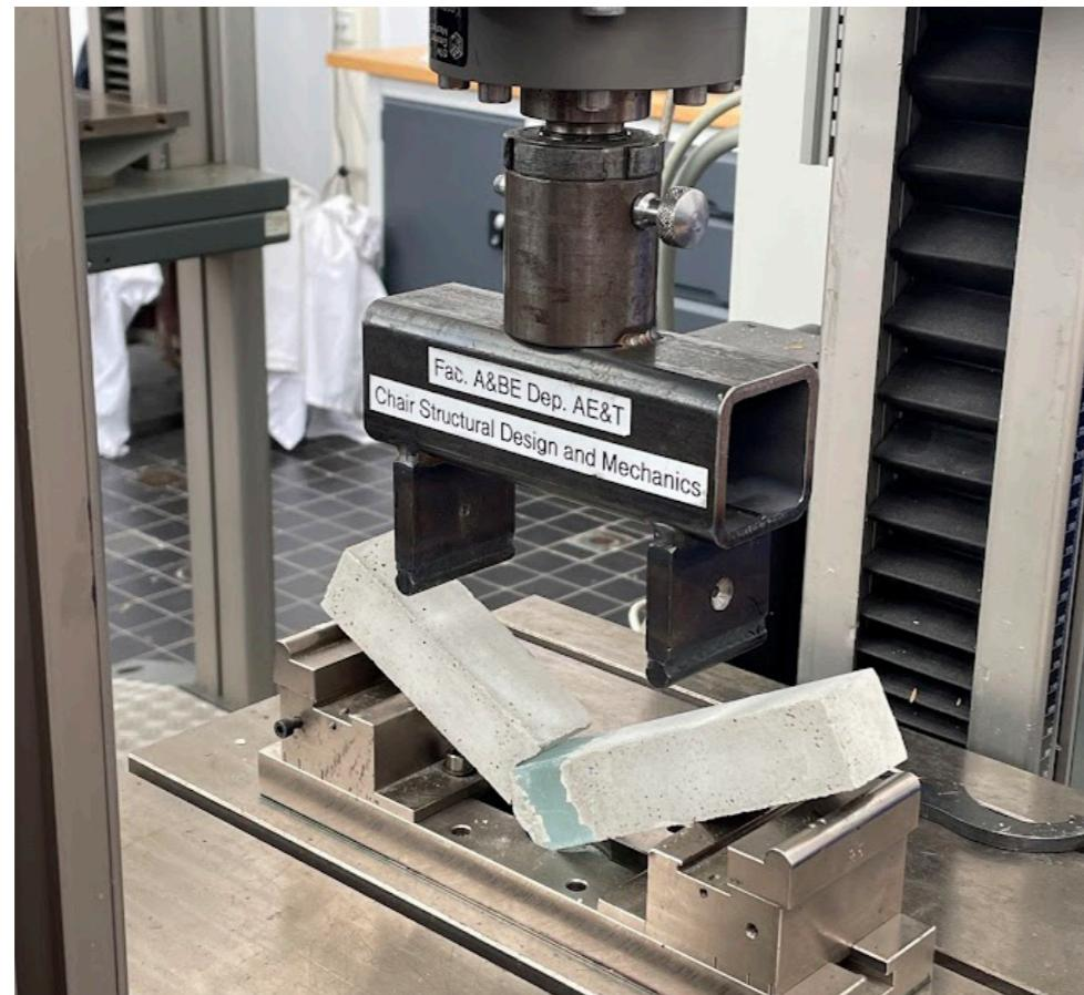
Four point bending test
