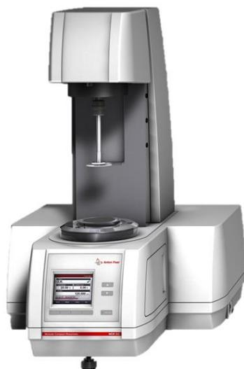
Figure 3-7: The Anton Paar MCR302 rheometer used for the rheology study
