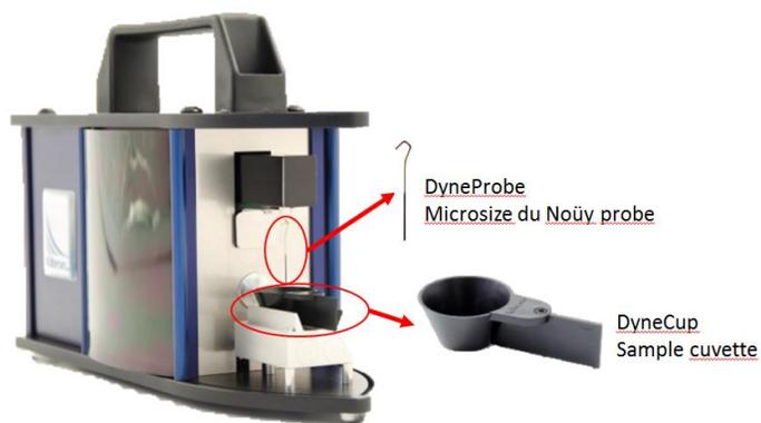
Figure 3-2: Kibron tensiometer used to measure the surface tension
