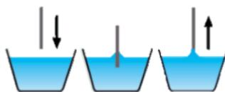
Figure 3-3: Du Noüy-Padday method for measuring the surface tension
